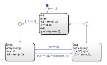
The chart consists of three states. At the start of simulation, the Init state initializes the chart data:
