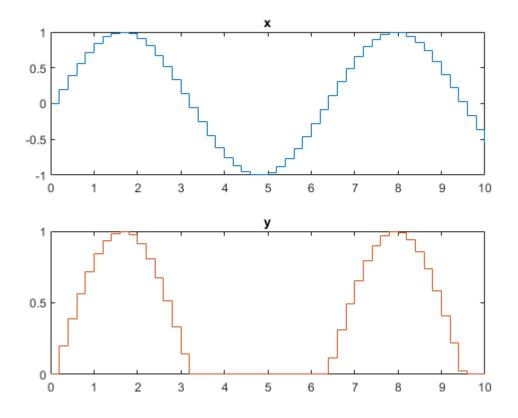
The execution results show that the rectifier filters out negative input values.
