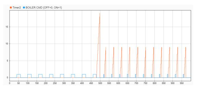
The shorter cycle and longer cooling time are a consequence of the substate hierarchy inside the On state. When the boiler reaches the reference temperature for the first time, the transition from HIGH to NORM keeps the controller on for an extra time step, resulting
