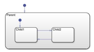
The contents of a parent state behave like a smaller chart. When a parent state becomes active, one of its child states also becomes active. When the parent state becomes inactive, all of its child states become inactive.
