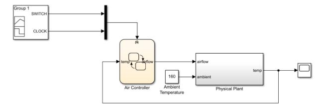
Based on the air temperature temp, the Air Controller chart turns on the fans and passes the value of airflow to the Physical Plant subsystem. This output value determines the amount of cooling activity, as indicated by this table.
