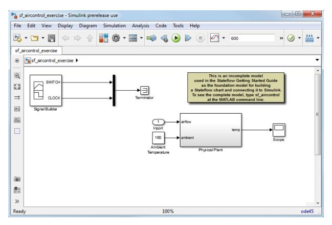
The model is incomplete because it does not include the Stateflow chart that you will build as you work through the exercises in this guide. Instead, the model contains several nonfunctional blocks: the Terminator, Inport, and Annotation blocks.
