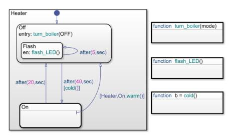
The actions guarding the transitions between the  ${\tt On}$  and  ${\tt Off}$  substates define the behavior of the bang-bang controller.
