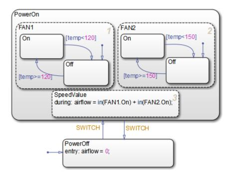
Now that you have associated these transitions with the event SWITCH, the control system will alternately power on and off every time SWITCH occurs — that is, every time the chart detects a rising or falling signal edge.
