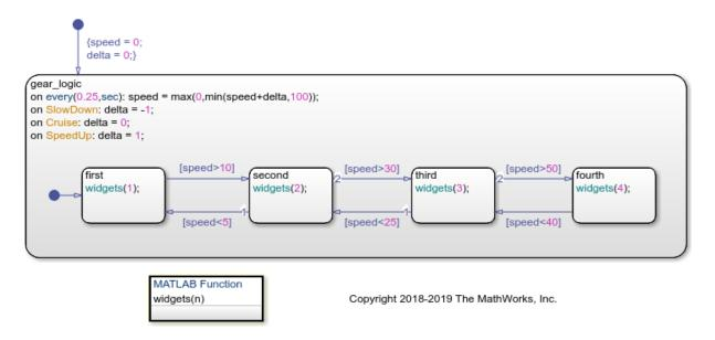
You can execute this chart as an object in MATLAB directly through the Command Window or by using a script. You can also program a MATLAB app that controls the state of the chart through a graphical user interface. For example, this user interface sends an input event to the chart when you click a button. In the chart, the MATLAB function widgets controls the values of the gauges and lamps on the interface.
